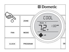
1. To turn ON the CCC 2 thermostat when the back light is off, first press any button to wake up the CCC 2 thermostat. Then press and release the **ON/OFF** button.
