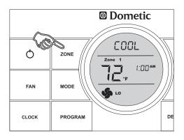
3. Press the **ZONE** button to cycle through the available zones to be programmed. Each zone signifies a unit designated to cool, heat or dehumidify a specific area of an RV. The Dometic Comfort Control Center 2 thermostat can control up to four units (zones).
