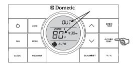
8. Press and hold the **OUTSIDE TEMP** button and the LCD will display the current outside temperature recorded at the outdoor temperature sensor in place of the temperature set-point. The LCD will also display "**OUT**" to indicate the outside temperature is being displayed. When the **OUTSIDE TEMP** button is released, the LCD will return to the programmed temperature set-point.
